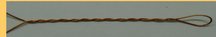
Insulation varnish coated coil prototype
