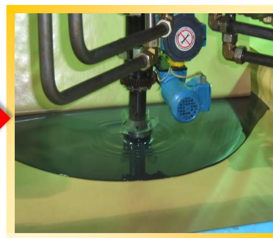
Foaming (Checking the Raw Liquid Flow and Foam Formation)
